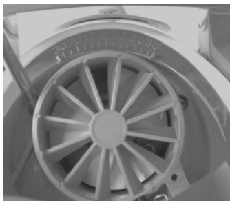
7.1: Remove the flap assembly to clean the dirt or hair on impeller
