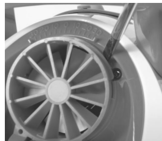
7.2: Use a flat screw driver to pry the flap assembly out as shown
