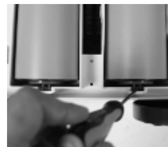
8.2: If the debris are not easy to access, use a flat screw driver to temporary remove the rollers. Push tab as shown in picture to remove.
