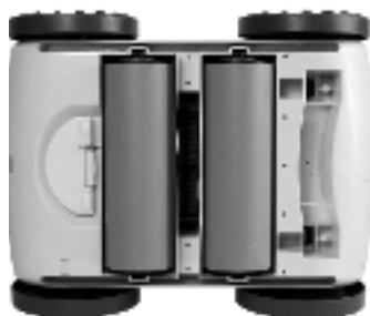
8.1: Manually rotate the green rollers. They should turn easily. If debris is blocking the rotation, remove the debris
