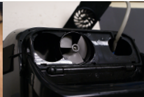
7.2 Clean the impeller. 7.3 Replace the grill guard.
